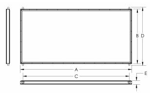
95%/5% Absorbtivity/Emissivity: Absorber Plate Aluminum 1" Nominal Copper (1.125" OD) Header Size: Riser Size: 3/8" Nominal Copper (0.50" OD) Glazing: Low Iron Prismatic/Matt Tempered Glass Glazing/Header Seal: **EPDM** Frame: AA 6063-T6 Bronze Anodized Aluminum **Backing Plate:** AA3105-H26 Painted Embossed Aluminum Insulation: Polyisocyanurate and Fiberglass R>12
